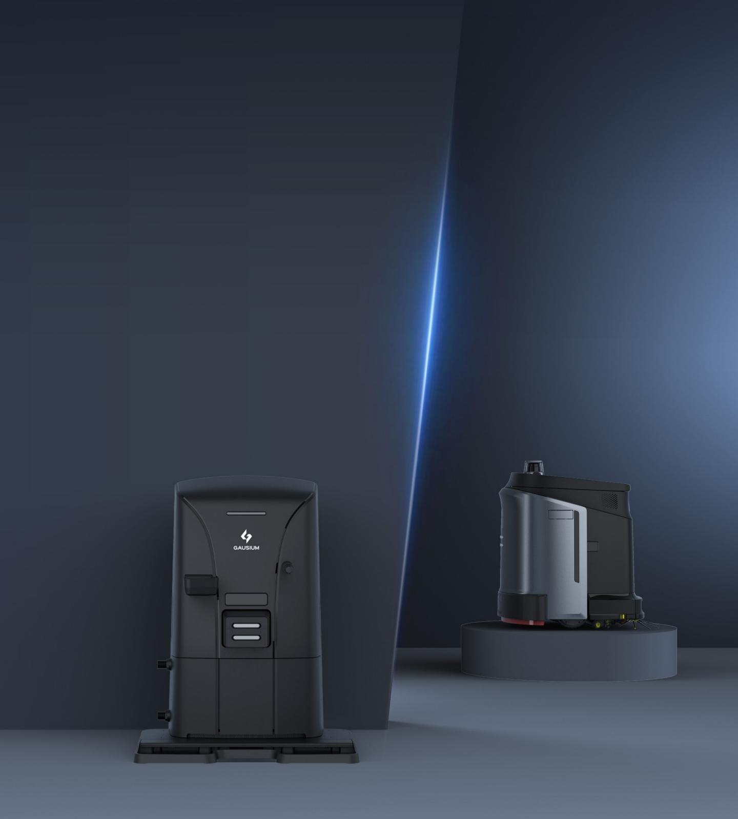
to maximize uptime and minimize human intervention, the WS-03-S allows the robot to automatically perform essential tasks such as power charging, water refilling, and discharge by simply docking with the workstation.
